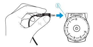
Connect the 3.5 mm jack plug of the headphones to the socket 5 of the receiver.
